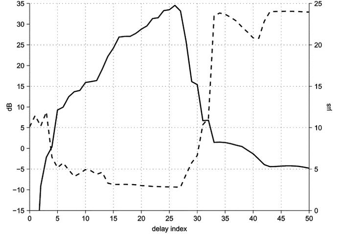
Fig. 3. SSNR (solid) and delay spread (dashed) obtained with the MSSNR design as a function of the delay index.
