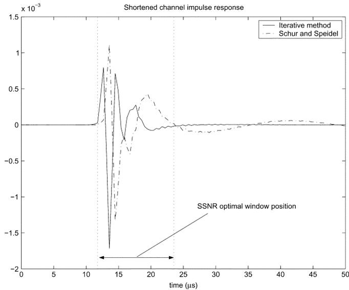
Fig. 4. Overall channel impulse response after shortening.
