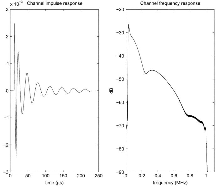
Fig. 2. Channel impulse and frequency responses.
