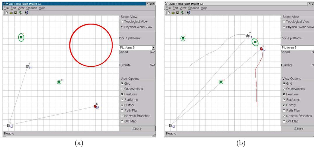
Figure 4: Human DDF node in action: (a) the operator enters a feature unknown to the sensor network and (b) the active nodes respond to its presence by converging onto it
