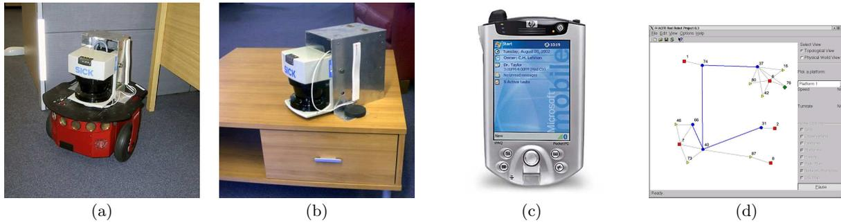
Figure 2: Elements of a practical decentralized ASN : (a) mobile platform (Pioneer II) with a mounted sensor (SICK laser range finder), (b) a stationary sensor (SICK laser range finder), (c) a mobile GUI node on an iPAQ PDA, and (d) a stationary GUI node on a Linux workstation
