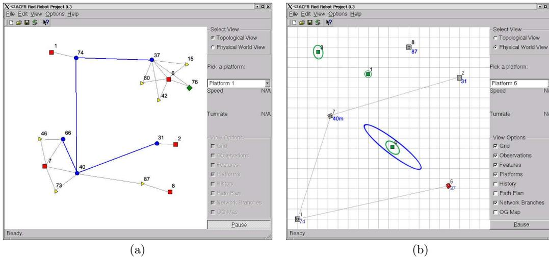
Figure 3: Two views of the same active sensor network: (a) topological and (b) physical. The topological view shows several ASN objects: platforms ( $\square$ ), nodes ( $\circ$ ), sensors ( $\triangle$ ), and controllers ( $\diamond$ ) with corresponding connections. The physical view shows mobile platforms connected by DDF links. Point features known to the network are also shown with corresponding covariance ellipses.
