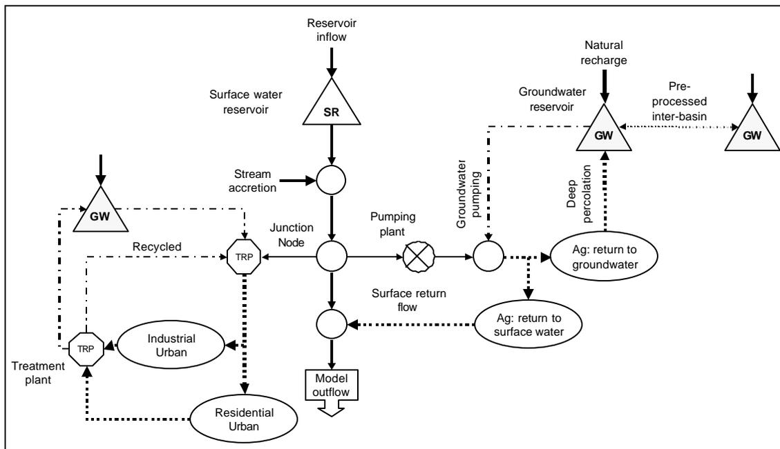
**Figure 2. Example network diagram for CALVIN**
