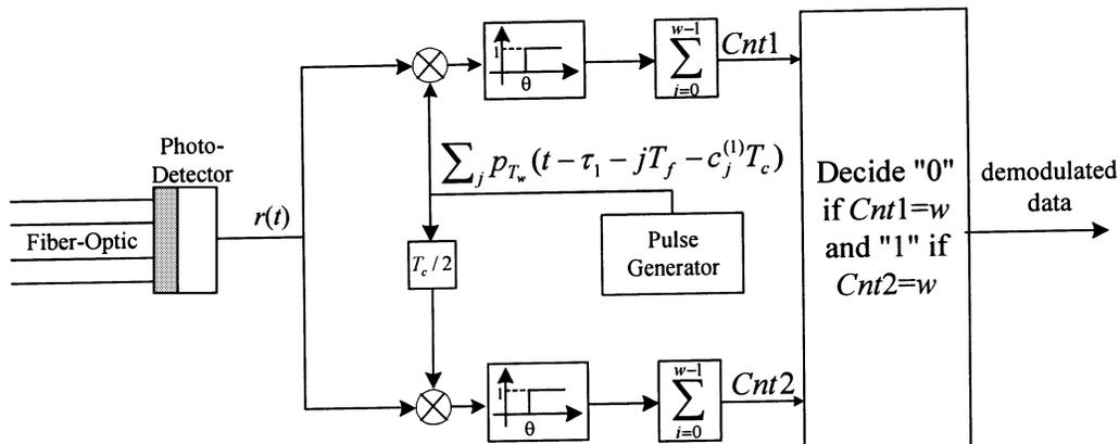
Fig. 4. Chip-level detector.
