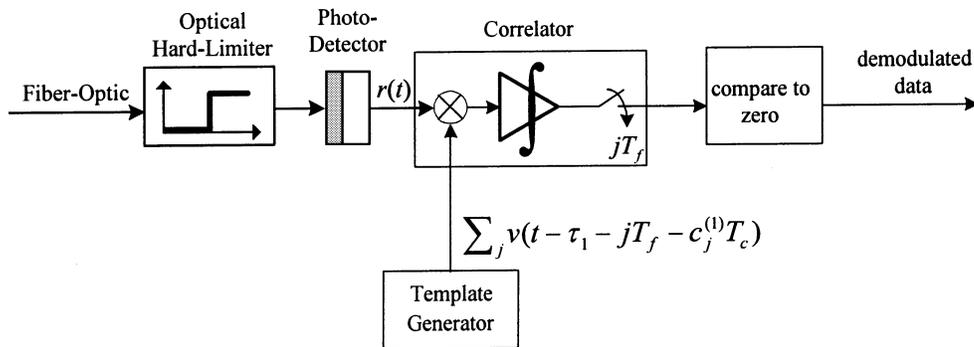
Fig. 3. Correlation receiver with an optical hard limiter.
