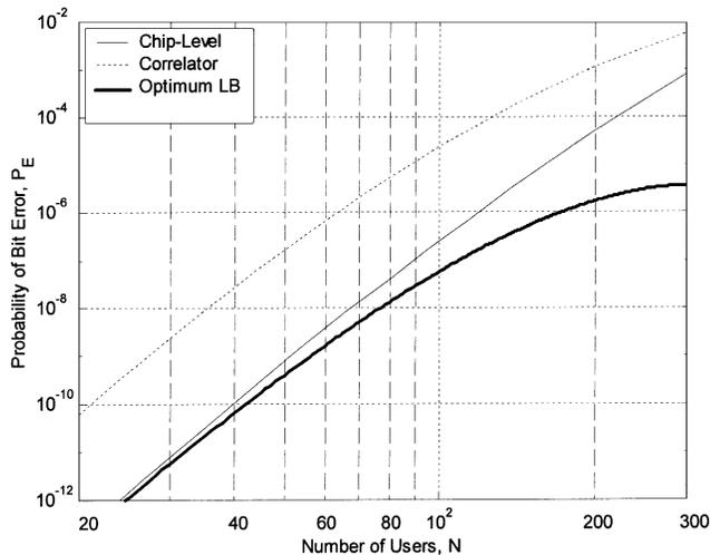
Fig. 9. Probability of bit error versus the number of users for various receiver structures with an ideal photodetector on a FTH system with  $F = 2000$  and  $w = 9$ . Note that with an ideal photodetector, the chip-level detector with optimum comparator threshold and correlation receiver with a hard limiter are the same as a chip-level detector.
