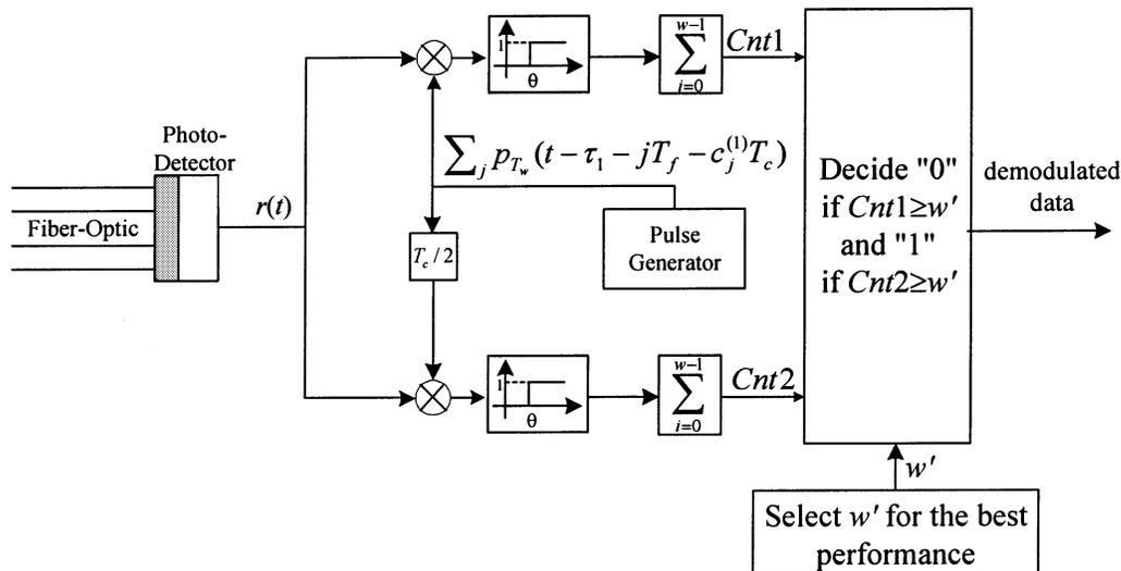
Fig. 5. Chip-level detector with optimum comparator threshold.
