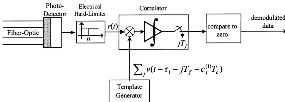
Fig. 6. Correlation receiver with an electrical hard limiter.
