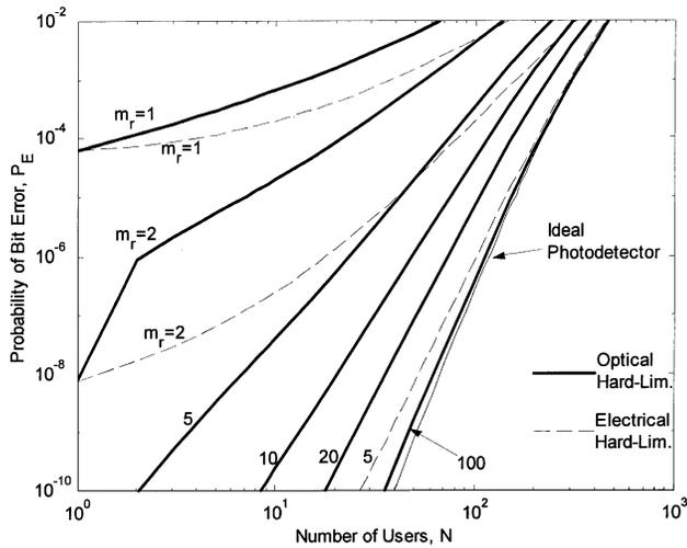
Fig. 12. BER of correlation receiver with an 1) optical hard-limiter and 2) electrical hard-limiter versus the number of users in various mean received photoelectron counts per pulse for a FTH system with  $F = 2000$  and  $w = 9$ .
