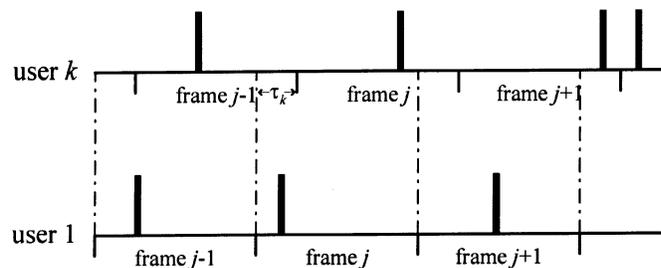
Fig. 7. Received pulse streams of user 1 and user  $k$ .
