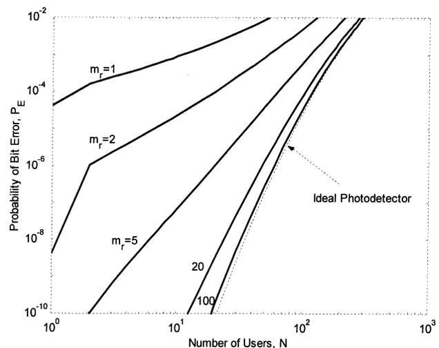
Fig. 10. BER of a correlation receiver on an FTH system with  $F = 2000$  and  $w = 9$  versus the number of users in various mean received photoelectron counts per pulse.
