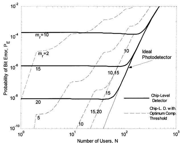
Fig. 11. BER of various receivers versus the number of users for an FTH system with  $F = 2000$  and  $w = 9$  in several mean received photoelectron counts per pulse.
