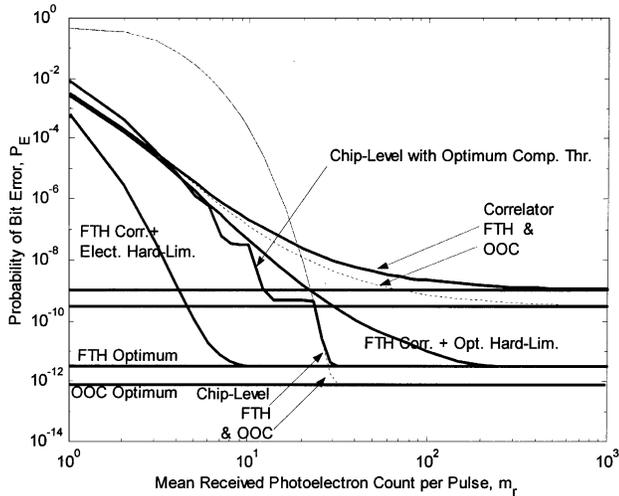
Fig. 8. BER of various receiver structures versus the mean received photoelectron count per pulse for FTH and OOC ( $\lambda = 1$ ) systems with  $F = 2000$ ,  $w = 9$ , and  $N = 27$ .
