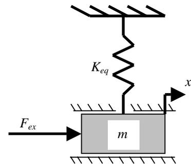
Figure 5. Mathematical model of the resonator
