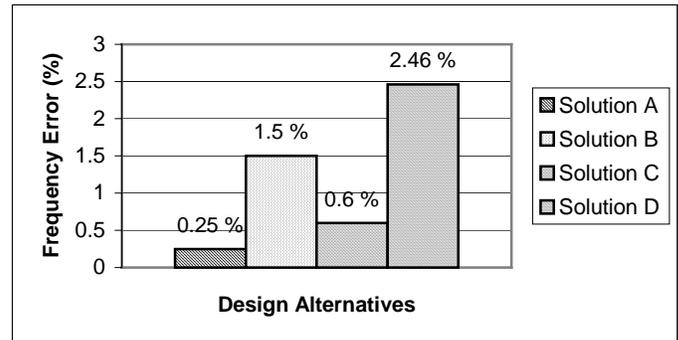
**Figure 9.** Design alternatives for a MEMS resonator categorized by frequency error %
