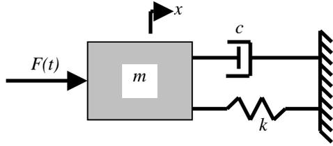
**Figure 1.** Lumped element model for a microresonator
