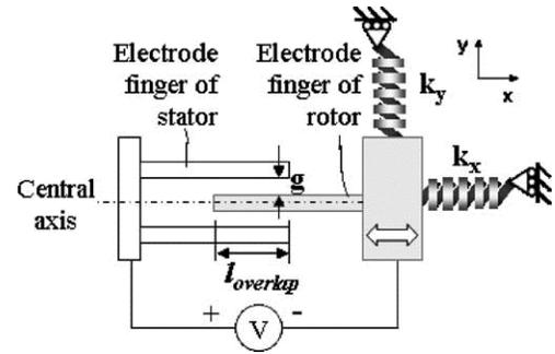
**Figure 2.** A Schematic diagram of comb drive actuator (Chen et al., 2004)
