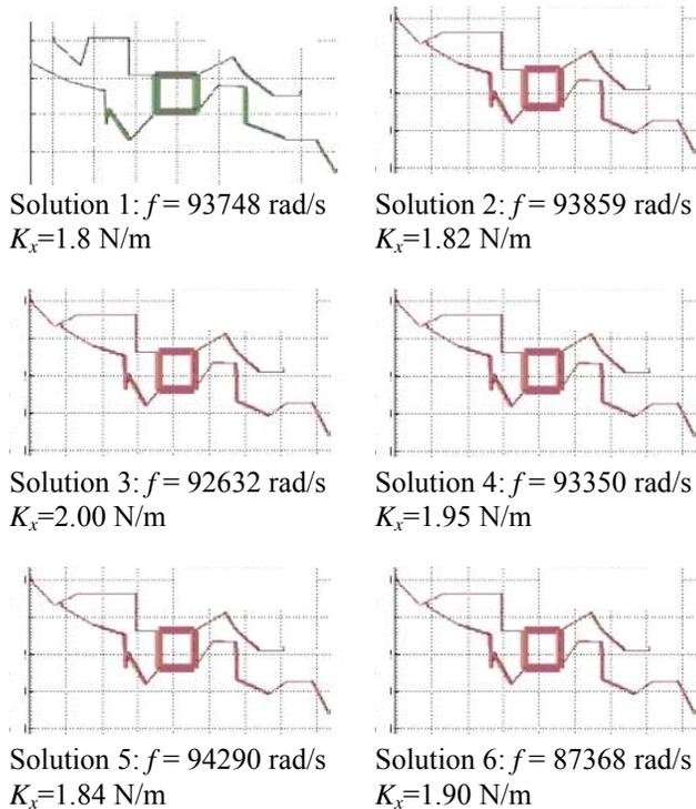
**Figure 11.** Design examples of meandering resonator (Zhou et al. 2002)
