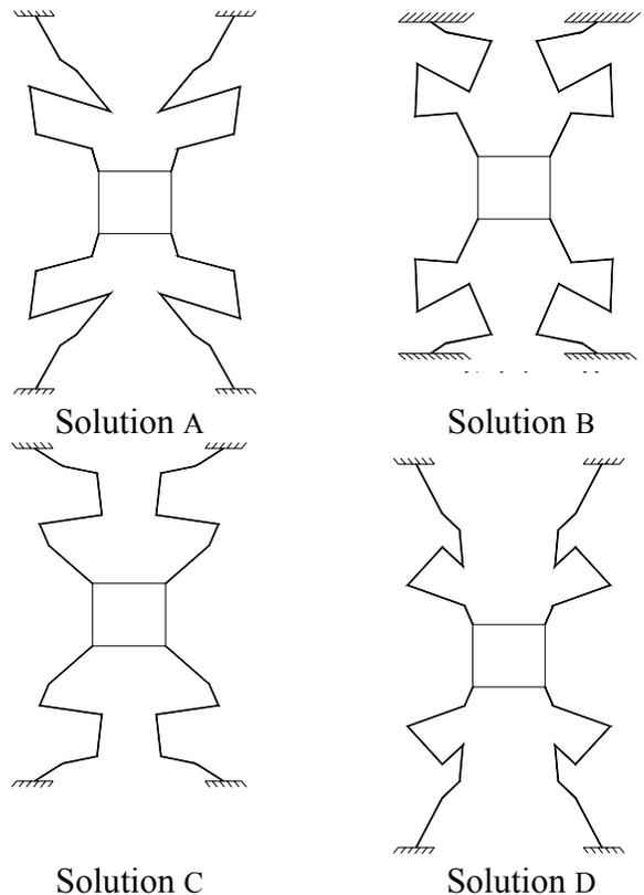
Figure 7. Design alternatives for a MEMS resonator
