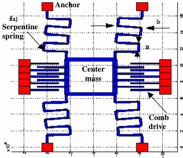
Figure 4. A MEMS resonator with four meandering springs (Kamalian et al. 2002)
