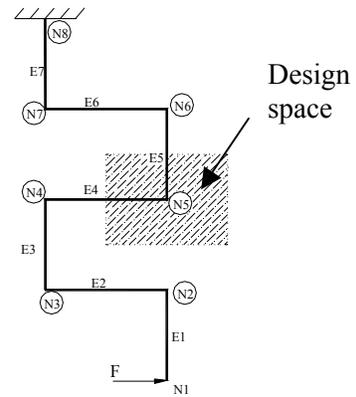
Figure 6. Design space for a MEMS resonator
