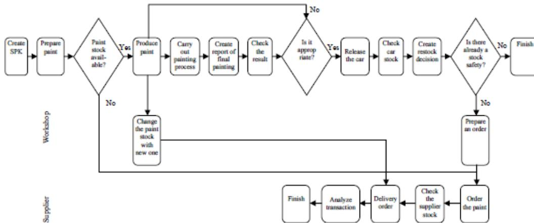
Figure-2. Process flow of To-Be scenario #1.
