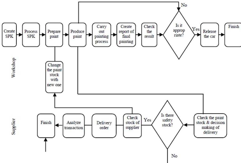
Figure-3. Process flow of To-Be scenario #2.
