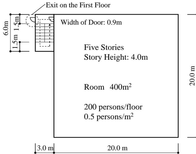
**FIGURE 8.** Plan of facility for case study
