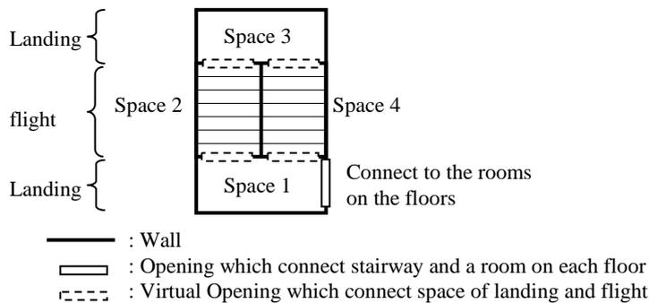
**FIGURE 3.** Modeling of space in staircase
