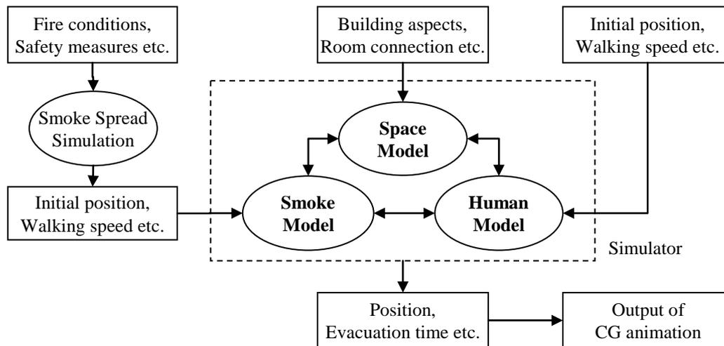
**FIGURE 1.** Composition of the simulation model
