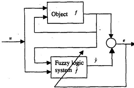
Figure 1. The serial-parallel identification model based on fuzzy logic system
