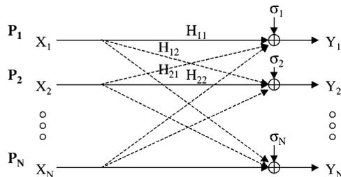
Fig. 2. A Gaussian interference network.
