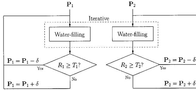
Fig. 5. A simplified illustration of the distributed power control algorithm based on iterative water filling.
