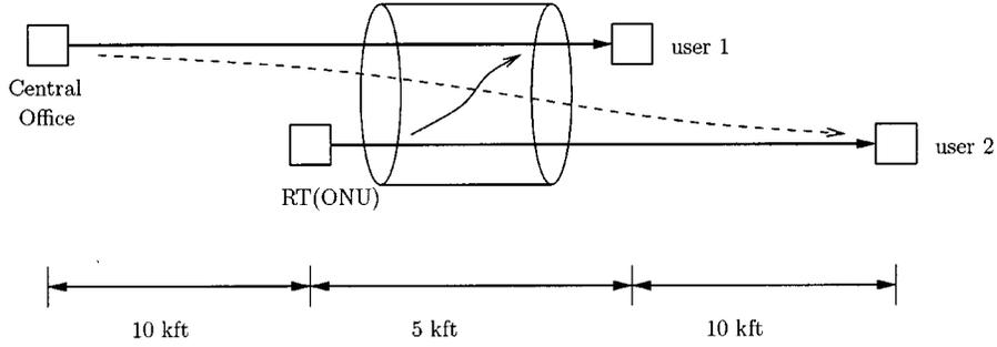
Fig. 10. CO-based ADSL versus RT-based ADSL.
