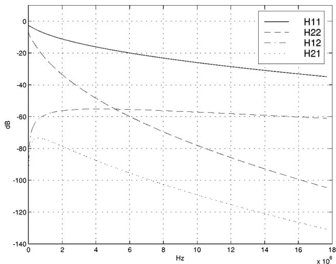
Fig. 6. Typical loop coupling and transfer functions: 3000 versus 1000 ft.
