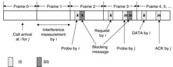
Fig. 3. The multiple access procedure.
