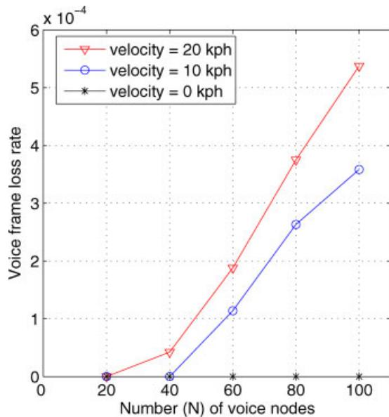
Fig. 5. The voice frame loss rate of a voice call.
