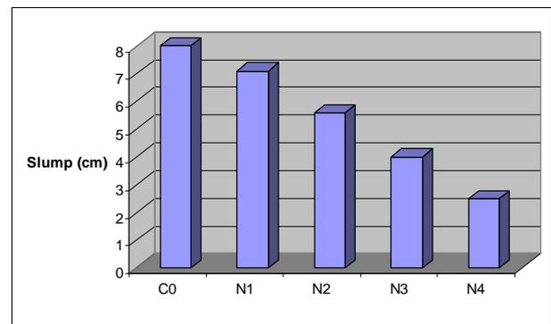
Figure 1. Particle size effects of nano- TiO<sub>2</sub> on workability of concrete. N1,N2,N3 and N4 are the series N blended concrete with 0.5, 1.0, 1.5 and 2.0 percent of nano- TiO<sub>2</sub> particles, respectively.
