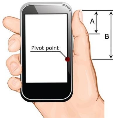
**Figure 2.** The thumb properties. A is the thumb tip length and B is the thumb length.
