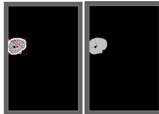
**Figure 4.** An example to demonstrate the image processing steps for an experimental record. The left shows the extracted center point by the bounding box method and the right shows the extracted center by the ellipse method.
