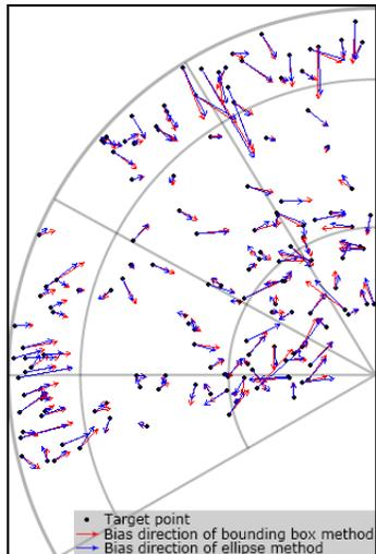
**Figure 6.** The directions of the touch biases, i.e. the directions from the target points to the extracted center points, for 144 experimental records.
