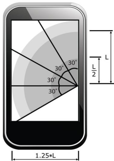
**Figure 1.** A touch surface can be divided by the angle conditions and the distance conditions.
