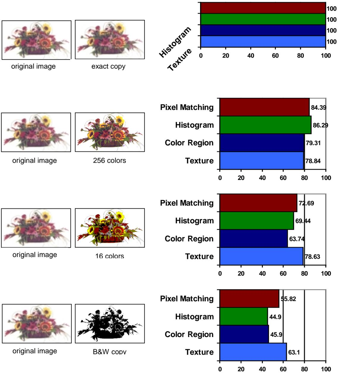
Figure A-3. Color Resolution Test
