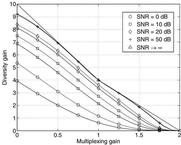
Fig. 4. Asymptotic and exact finite-SNR DMT for  $5 \times 2$  MIMO channel with solid lines and  $2 \times 5$  MIMO channel with dashed lines at various SNRs.
