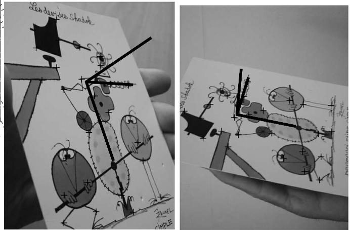
**Fig. 2.** Recovery of the 3D orientation of a reference plane from the single world-plane to image homography under the principal point constraint. The homography has been estimated from points represented with a white cross.
