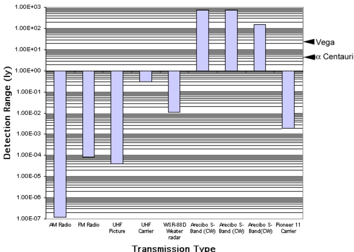
**FIGURE 3.** Log plot showing the detection range results for an Arecibo like-dish and various terrestrial transmission types assuming an Arecibo-like detector. The minimum detection range to receive a signal on Alpha Centauri and Vega is indicated with arrows.
