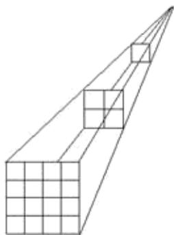
**Figure 2.** As electromagnetic radiation propagates outward into space, it is spread out over an ever increasing area.
