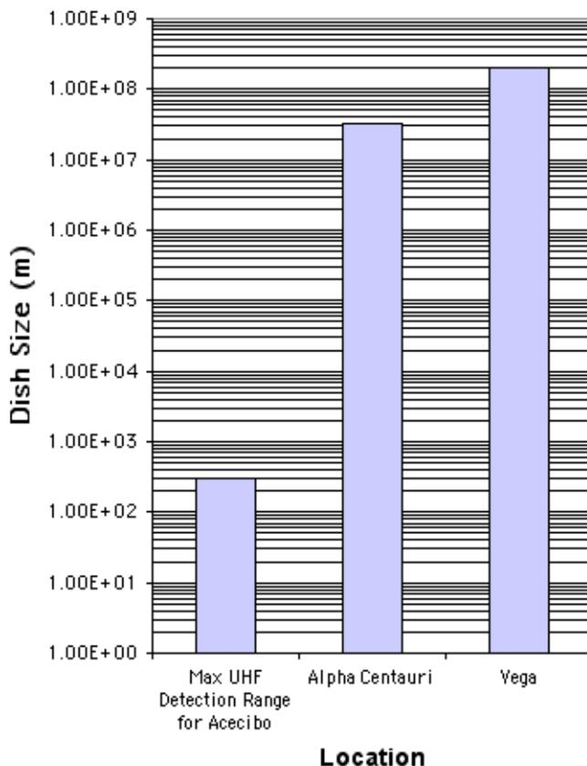
**FIGURE 4.** Log plot of minimum dish size required to receive a UHF signal leaked from Earth at various locations, assuming a receiving instrument similar to the Arecibo telescope.
