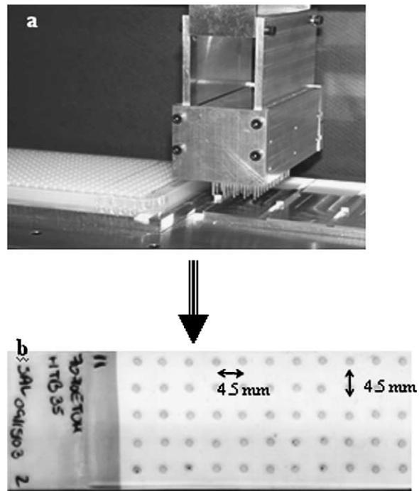
Fig. 2. (a) The automated cytology microarray depositing device. (b) The scan of a stamped and stained glass slide after preparation.
