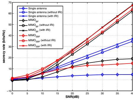
Fig. 2: Comparison of single-antenna with multi-user MIMO system
