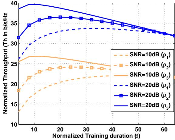
Fig. 4. Normalized throughput of the hybrid analog-digital channel estimation and beamforming for multiuser case.
