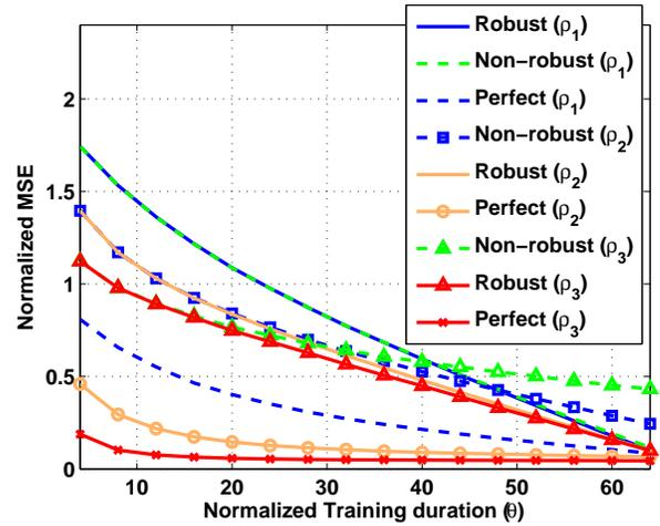
Fig. 6. Comparison of perfect, robust and non-robust hybrid analog-digital channel estimators.
