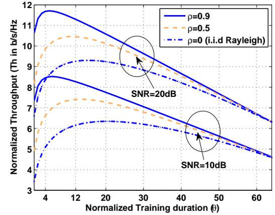
Fig. 3. Normalized throughput of the hybrid analog-digital channel estimation and beamforming for single user case.
