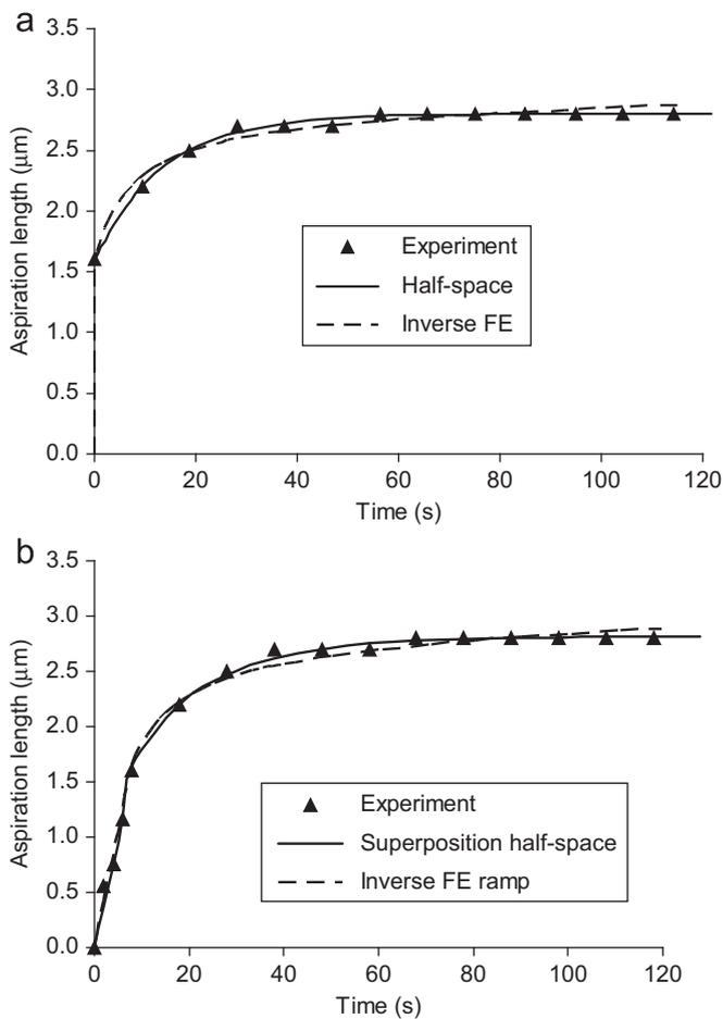
**Fig. 2.** The experimental deformation history of a typical VIC and the nonlinear regression curves determined by (a) standard half-space model and the inverse FE method assuming instantaneous loading; and (b) superposition half-space model and the inverse FE method under a linear ramp loading period of 8 s.
