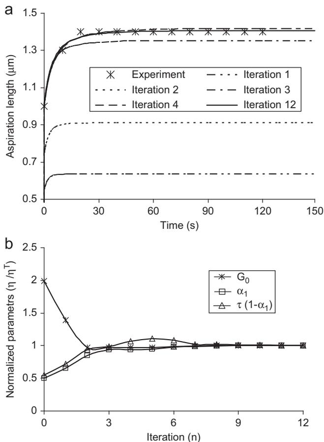
**Fig. 1.** Optimization process using the inverse FE method to analyze experimental data from one cell. The (a) initial, improved and optimized deformation history curves, and (b) convergence history are shown. Initial guesses correspond to those in the first three rows of Table 1.
