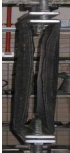
(a) whole tire with side walls removed being stretched until failure
