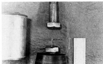
FIG 1.—Alastik module in process of being secured in specially designed grips.
