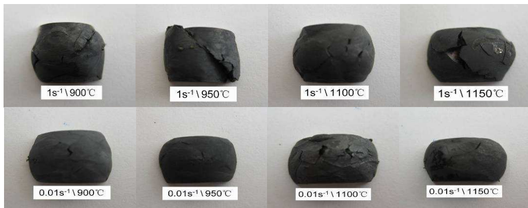
Fig.3 Cracking in as-cast state alloy, occurring at 1\text{s}^{-1} and 0.01\text{s}^{-1} , 50% reduction
