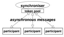
Figure 2. Reactive interpretation of rules. The synchroniser manages the pool of tokens internally.
