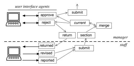
Figure 8. Relationships between tokens in the reporting example. The top half represents the manager's rules, the lower half the staff member's. The waitUntilNext and remove tokens have been left out for clarity.
