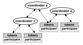
Figure 5. A tree of coordination. Coordinators a and b communicate via a shared participant, while coordinator c is a direct participant for coordinator a.
