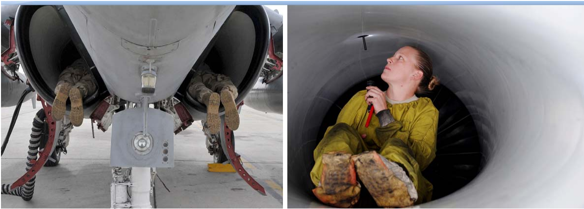
Figure 8. Inlet Inspection of E/A 6B and F-16. From [17]
