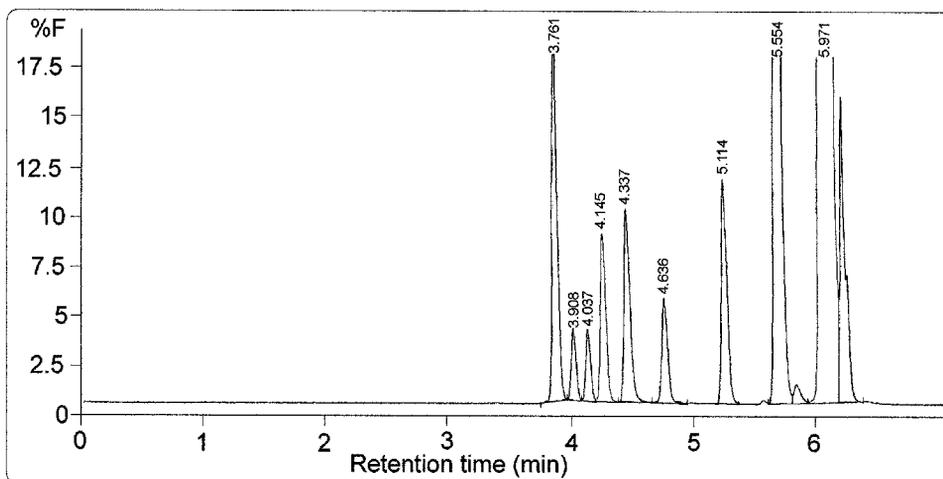
Fig. 1. Chromatograms obtained for calibration solutions containing 100  $\mu\text{mol/L}$  cysteine (3.761 min), 25  $\mu\text{mol/L}$  cysteinylglycine (3.908 min), 25  $\mu\text{mol/L}$  glutathione (4.037 min), 50  $\mu\text{mol/L}$  homocysteine (4.145 min), 50  $\mu\text{mol/L}$  cysteamine (4.337 min), and 50  $\mu\text{mol/L}$  MPG (5.114 min).
