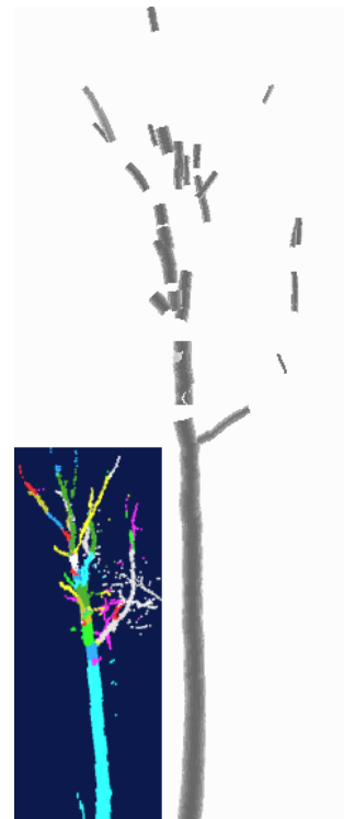
Figure 5: Automatic estimated branches of a leaf tree. The inserted shows the result of the segmentation in voxel space, the large image shows the reconstructed branches.
