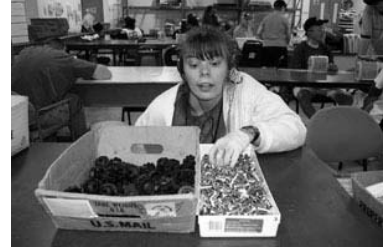
Cara McCricker assembles sound isolation clips at Oppor- tunity Village in Las Vegas.
