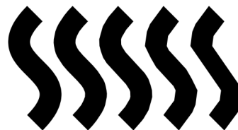
Figure 9: Splines drawn with tolerance values of .1, .5, 1, 5, and 10
