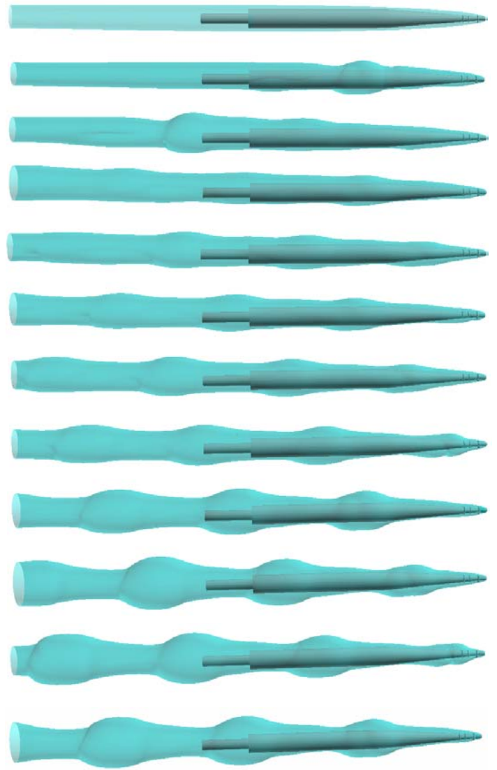
Figure 6: Cavity evolution from initial condition to periodic wave shape effected by planing limit cycle. Snapshots from (tU_0/L)=0 through 5.73 shown at regular intervals of duration 0.5208. Cavity illustrated by isosurface at \rho_L=500.\text{kg/m}^3 .
