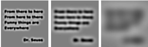
Figure 3. Difference of Gaussians: f_s - f_{3s/2} , s = 8, 16, 44 . 50% gray is zero; dark gray is negative; light gray is positive.
