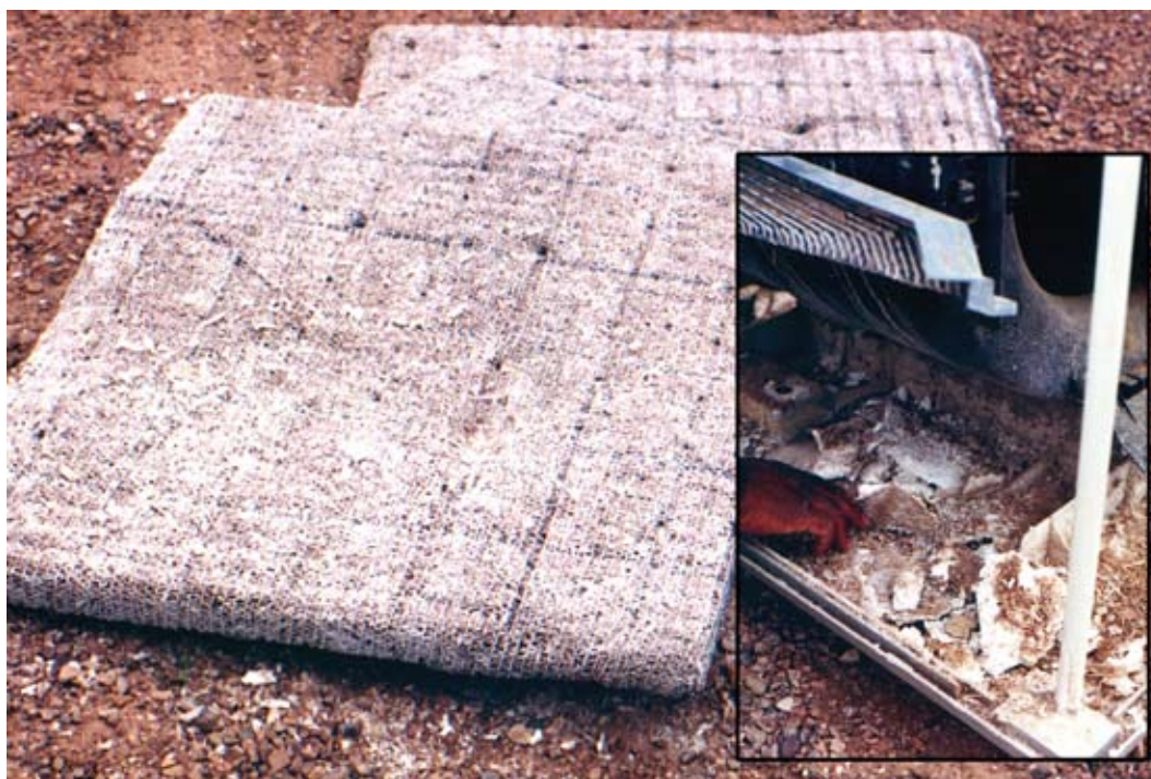
Figure 5.5: The build-up of salts on and below evaporative cooling filters at a house in Nepabunna
