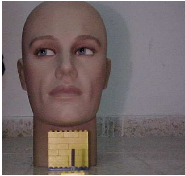
Figure 17: The imaged object and the calibration accessories: the illumination direction is derived from the position of the shadow of the vertical rod on the lego wall.
