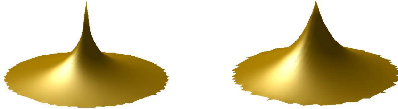
Figure 5: Left : In the discrete case, straightforward use of a control point as a constraint in computing depth from normal directions creates a tent-pole. Right : Reconstruction using the Terzopoulos formulation. In both cases, as dictated by the control point, the height of the peak above the base plane is 1.
