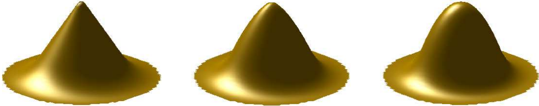
Figure 7: Left: Reconstruction with w(\tilde{r}) = 1/\tilde{r} . Middle: w(\tilde{r}) = 1/\tilde{r}^{1.5} . Right: w(\tilde{r}) = 1/\tilde{r}^2 . Here \tilde{r} = \min\{r, R - r\} ; the reconstructed surface complies with the gradient field data near the perimeter of \mathcal{D} . In all three cases, as dictated by the control point, the height of the peak above the base plane is 1.
