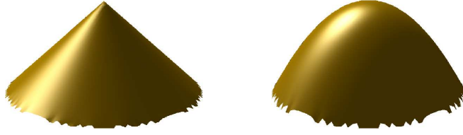
Figure 6: Left : Shape recovery with w(r) = 1/r for the example discussed in subsection 2.2. Right : w(r) = 1/r^2 . The difference between the two cases is in the distribution of the discrepancy between the gradient field data and the reconstructed gradients within the domain \mathcal{D} , necessary in order to comply with the hard constraint z(0,0) = 1 . In both cases, as dictated by the control point, the height of the peak above the base plane is 1.
