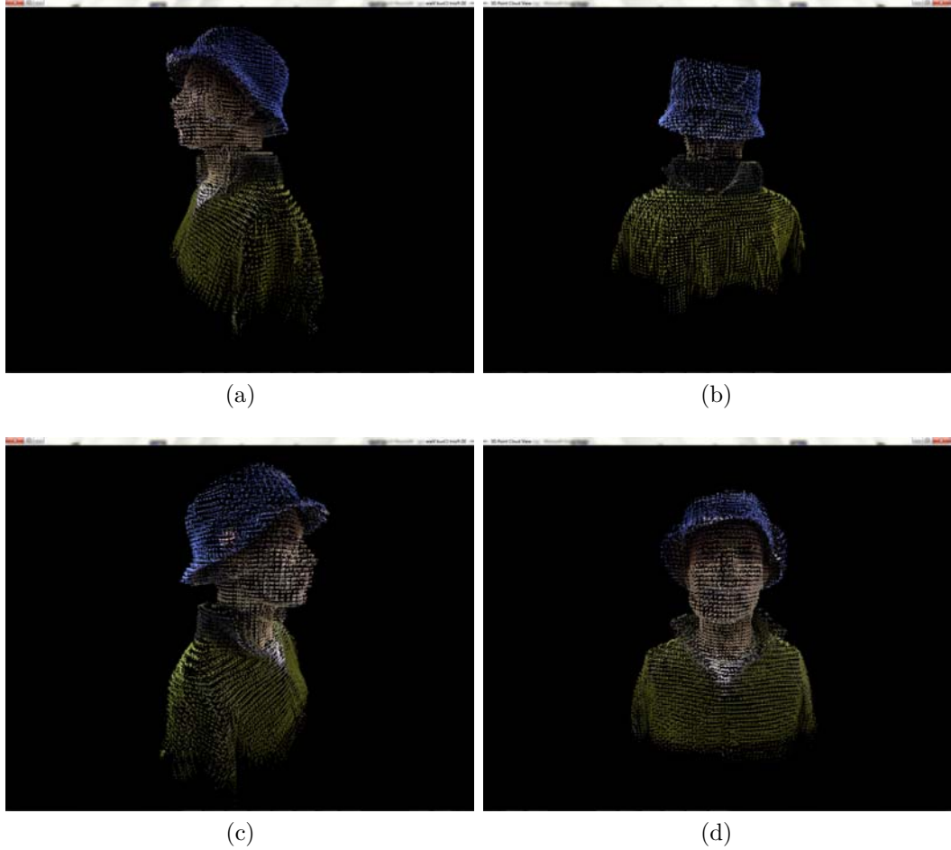
Figure 5.4: The dummy 360° scanning: a) Camera passing \frac{1}{4} circle. b) Camera passing \frac{1}{2} circle. c) Camera passing \frac{3}{4} circle. d) Camera passing one circle. The Camera moves in the counterclockwise direction
