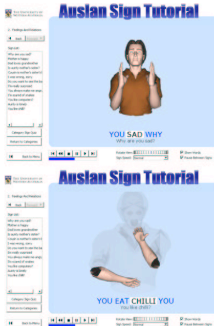
Figure 8. Some screen shots from the Auslan Tuition System showing the graphical interface. The top image shows the avatar with a sad expression while signing the phrase “Why are you sad?” The bottom image shows the transparency used when viewing from a pseudo first person perspective which occurs when the avatar is rotated 180 degrees.
