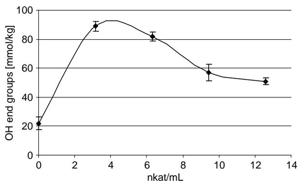
Figure 4. Hydroxyl groups in PET after treatment with different activities of the *T. lanuginosus* enzyme preparation. Error bars show the standard deviation of the measurement carried out in triplicate.
