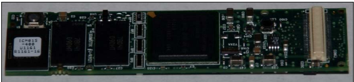
Fig. 10. gumstix connex TM ; view of processor in middle of board.
