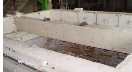
Fig. 2 Specimen installed on the horizontal heating furnace
