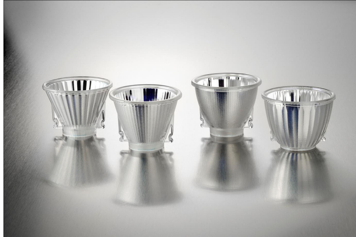
Figure 4: Reflectors with beam angles of 10, 15, 25 and 40 degree. The outer dimensions are identical for all types. All structures needed for the reflector mounting are already pressed in during the hot-forming process.
