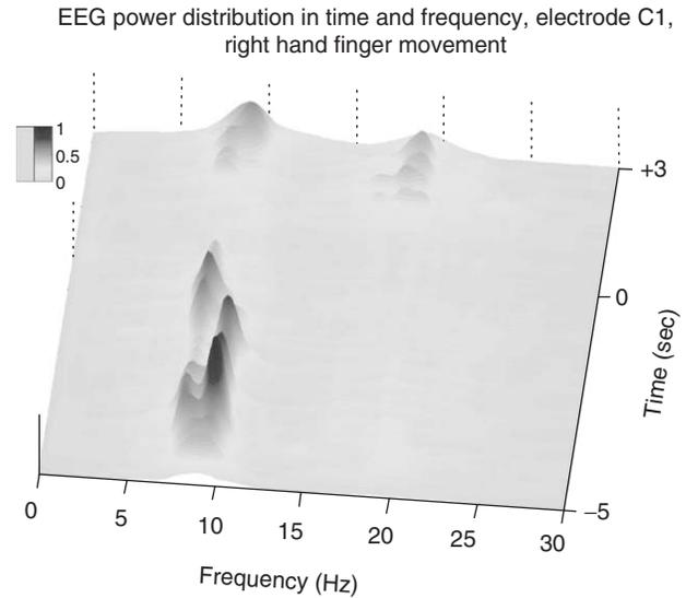
**Figure 7.** EEG power distribution in time and frequency during voluntary finger movement (movement onset at time 0) for electrode placed above sensorimotor cortex. The desynchronization (decrease of amplitude) is visible for alpha and beta band before the movement and their synchronization may be observed after the movement. (EEG filtered in 0.5–100 Hz frequency range. The power was divided by 1/f in order to suppress the frequency-dependent background.)
