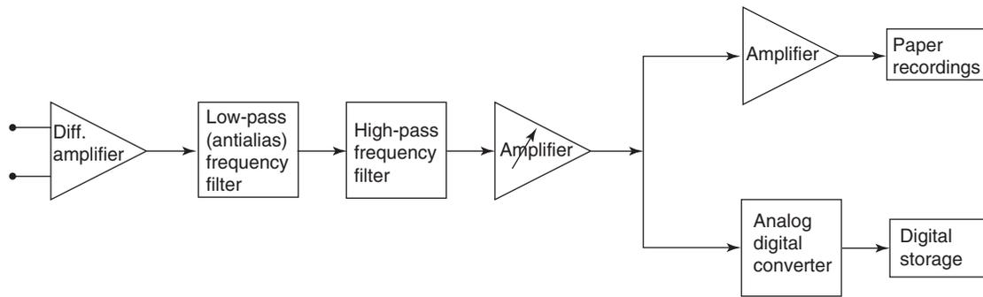
**Figure 4.** Block diagram of recording of a single EEG channel. Differential amplifier measures potential between two electrodes (one of them is treated as the reference). Analog filters and adjustable amplifier prepares the signal for analog-digital conversion (ADC) and storage (lower path). Before the proliferation of digital media, EEG was stored on folded paper (upper path).
