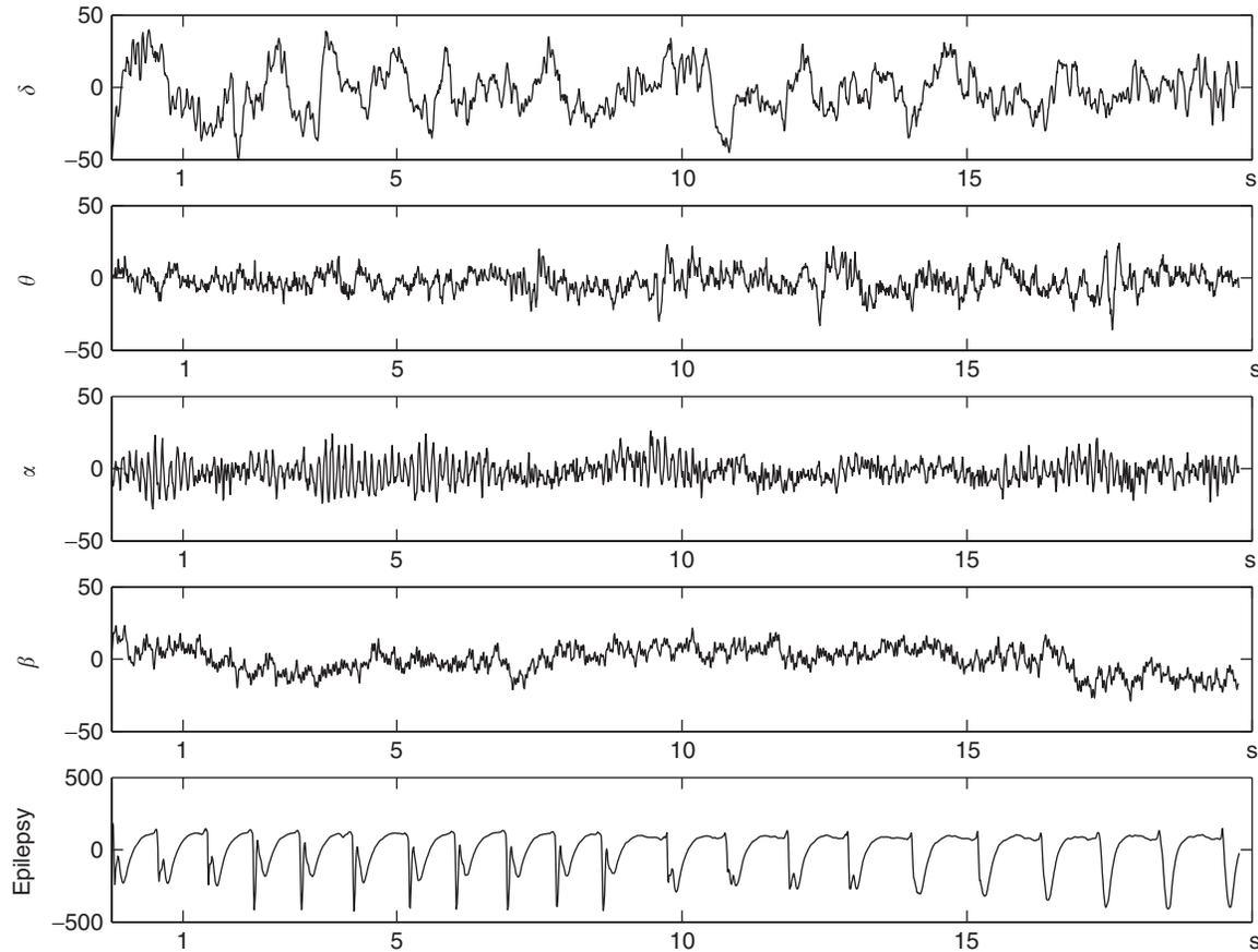
**Figure 1.** Characteristic EEG rhythms, from the top:  $\delta$  (0.5–4 Hz),  $\theta$  (4–8 Hz),  $\alpha$  (8–13 Hz),  $\beta$  (13–30 Hz). The lowest trace—EEG during epileptic seizure, note that the amplitude scale is an order of magnitude bigger.
