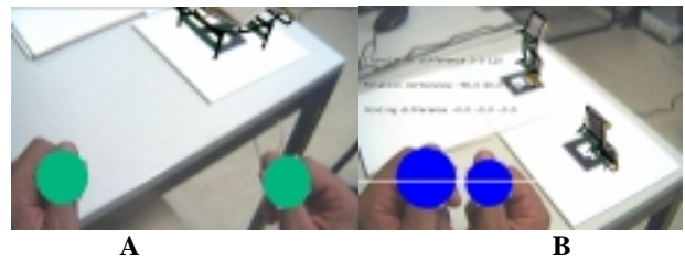
Figure 9 Rotation test on the near object (local YY' axis): A - The user first sets the desired axis with a gesture; B - Subsequently, the user issues a circular motion with both hands, as if turning a vertical steering wheel and within the boundaries of a displayed circle.
