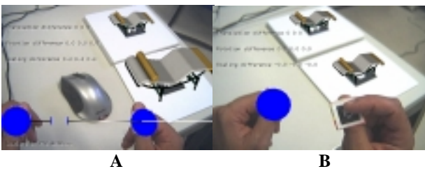
Figure 8 Scaling test on the near object: A – Tangible interaction; B – Terminating the Tangible interaction by occluding the Magic Ring with the index finger.
