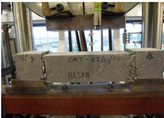
Fig. 9: Illustration of fibrous beam after direct shear test
