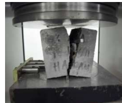
Fig. 6: Plain concrete after tensile test
