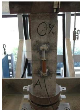
Fig. 3: Load vs. deformation test set up
