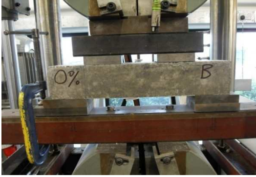
Fig. 2: Instrumentation of beam specimen for direct shear test
