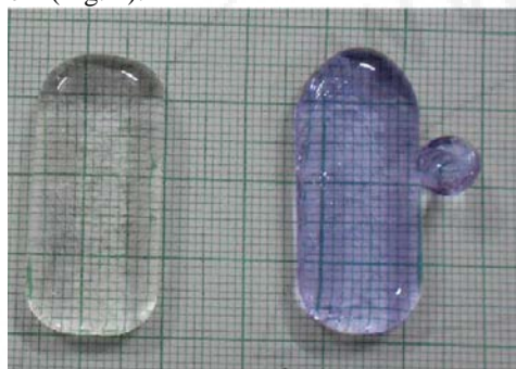
Fig. 1 Images of pure and doped glasses of the \text{Li}_2\text{O}-\text{Al}_2\text{O}_3-\text{P}_2\text{O}_5 glass system
