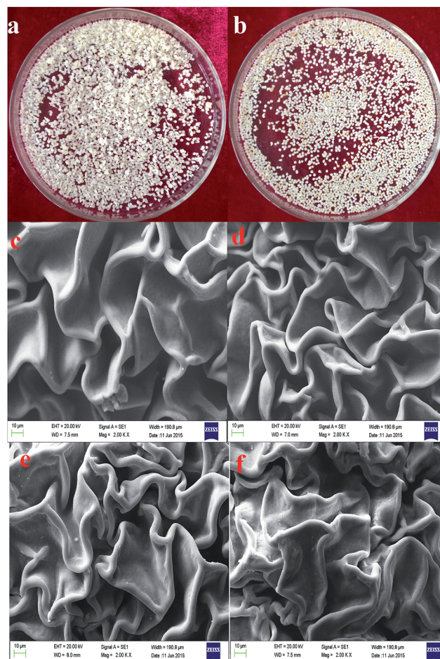
Fig. 1 Photos and SEM images of adsorbents ((a) digital photo of CMC-La, (b) digital photo of linked-CMC-La, (c) SEM of CMC-La, magnification \times 2000 , (d) SEM of linked-CMC-La, magnification \times 2000 , (e) SEM of CMC-La after adsorption, magnification \times 2000 , (f) SEM of linked-CMC-La after adsorption, magnification \times 2000 ).
