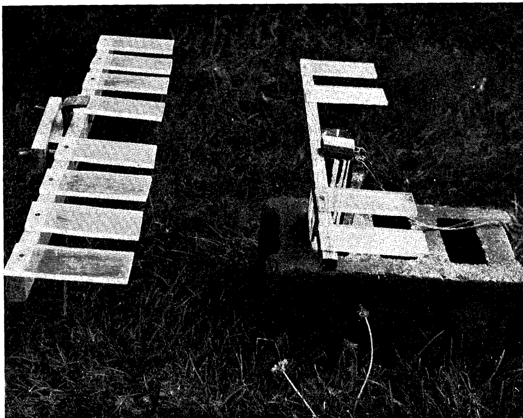
FIG. 1. Plexiglass substrata and supporting devices used for the collection of stream periphyton.
