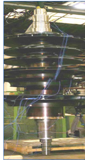
Figure 15. Ethylene rotor undergoing modal testing.
