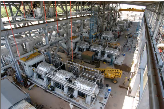
Figure 14. Photograph of compressor deck showing the six compressor strings. From front to back- 2 x methane compressors, 2 x ethylene compressors and 2 x propane compressors.
