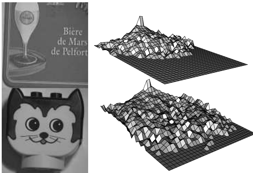
Fig. 2. Two-dimensional histograms of two objects corresponding to a particular viewpoint, image plane rotation and scale. The image measurement is given by the Magnitude of the first derivative and the Laplace operator. The resolution of each histogram axis is 32.
