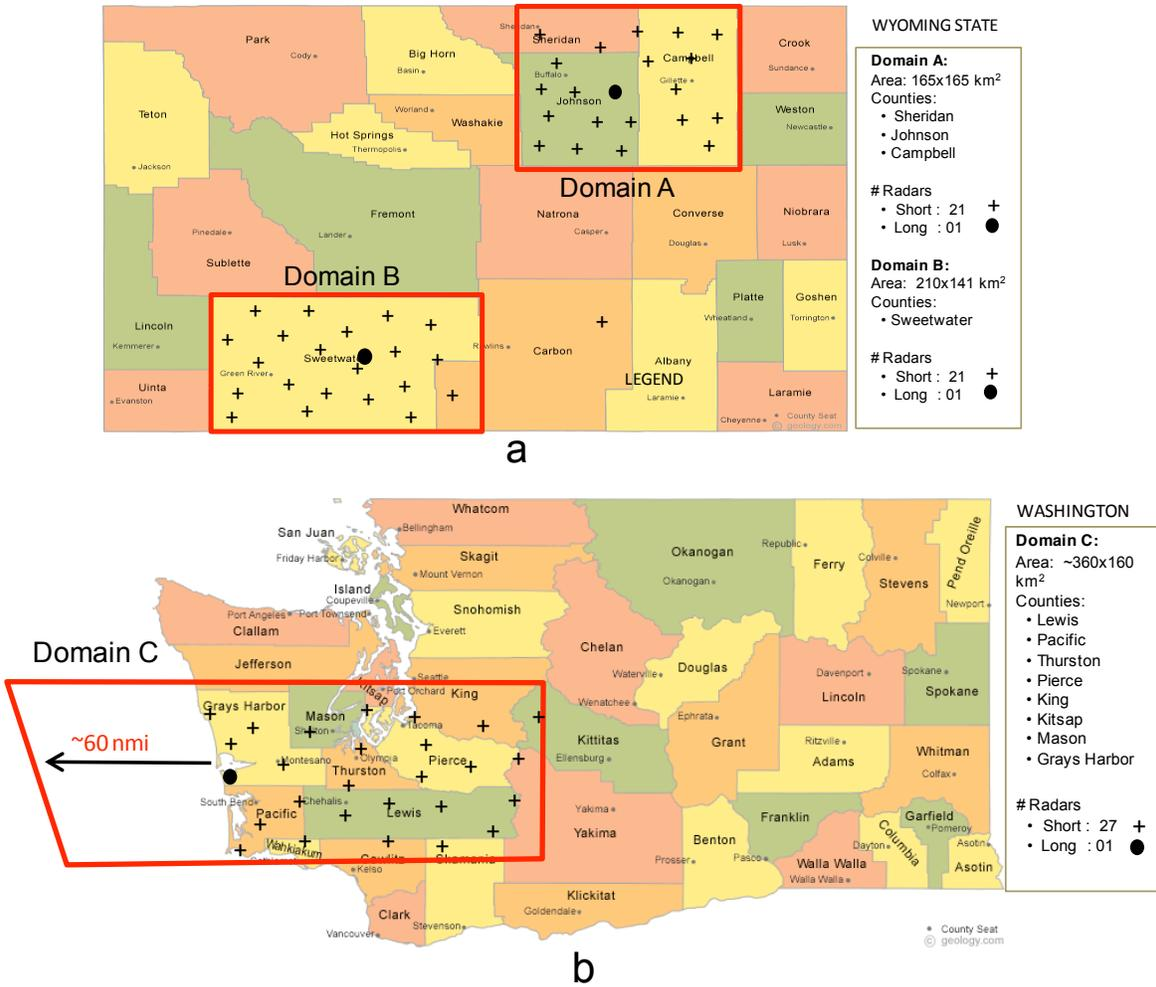
Figure 6.5: Potential long-range (large circle) and short-range radar locations (crosses) for a) Wyoming Domains A and B and western Washington Domain C.
