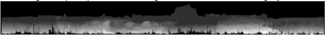
Figure 6. Panoramic depth map generated from stereo images.
