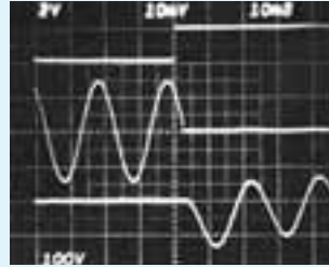
L load (2.5-A pure inductive load)
